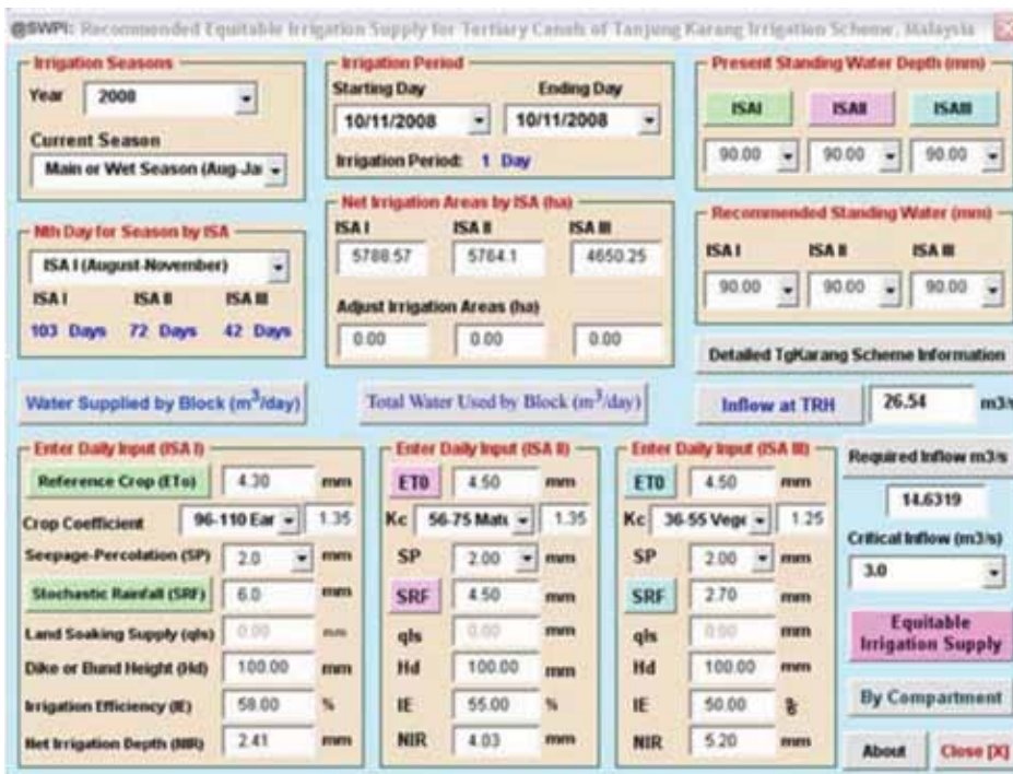
Fig.5: Dialog Wizard for Recommended and Equitable Irrigation Water Allocation by Tertiary Canals, 10 November 2008
